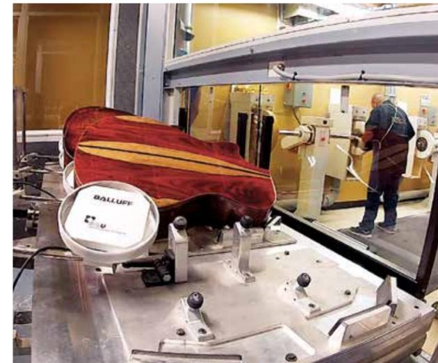
Pallet drawers where bodies are loaded for buffing. The round casing holds an RFID scanner
